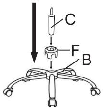
**STEP 2:**Attach the metal cover F on top of the spider base B then insert the gas lift C to the center hole of the base B.
