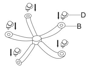
**STEP 1:**Insert casters D to bottom of the spider base B.
