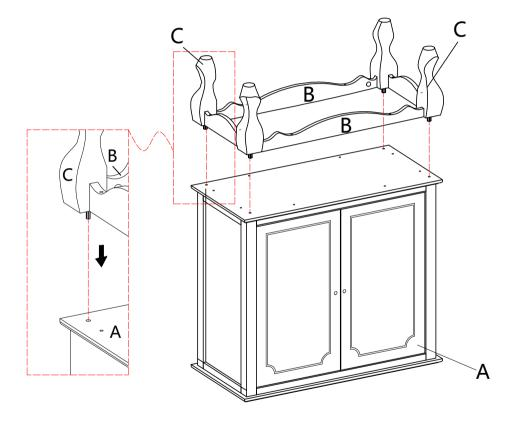
In preassemble step 3, make sure all holes aligned and then use bolt #4 to attach them, tighten bolt #4 with screwdriver #12.
