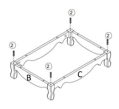
**STEP 3:**Insert dowel #2 on leg part B once part B&C assembling completed.
