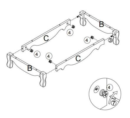
**STEP 2:**Use philips head screwdriver #7 to fasten cam lock #4 for secure part B & C.
