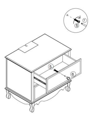
**STEP** 6:Use philips head screwdriver #7 to fasten bolt #5 & knob #6 on drawer front panel.
