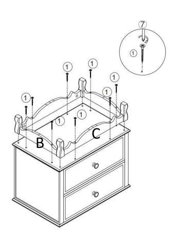
**STEP 4:**Insert screw #1 on part B&C,use philips head screwdriver #7 to fasten it.
