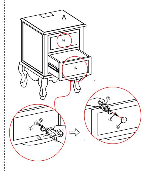
**STEP 5:**Remove the screw using #⑦ screwdriver, place the handle in front of drawer panel, connect the handle with a screw and lock the screw with a screwdriver#⑦.
