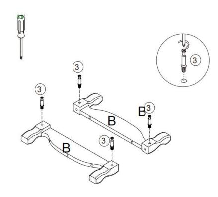
**STEP 1:** Use philips head screwdriver #7 to fasten cam bolt #3 on leg part B.
