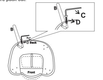
STEP 2: Use bolt D, allen key C to attach legs B to bottom of the seat/back A.
