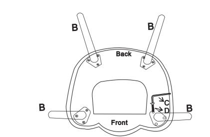
**STEP 3:** Use bolt D, allen key C to attach legs to bottom of the seat/back A. Make sure all parts align then fasten all bolts to secure.
