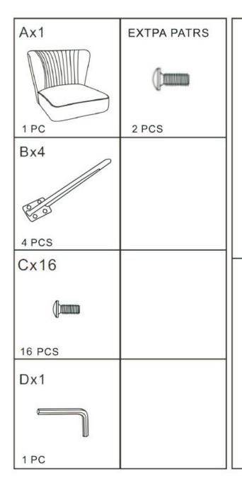
1 Place the Chair Back A on a clean padded surface. Use bolt C, allen key D to connect the metal leg B to bottom of the seat cushion A, make sure all holes algin, fasten all bolts to secure.
